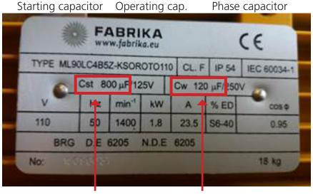
Cst = 800uF Starting capacitor Cw = 120uF Operating capacitor Gear motor plate, 110V, 1.8kW fitted with just 2 capacitors the starting- and operating capacitor = 120 L
