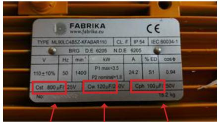
Gear motor plate, 110V, 1.8kW fitted with all 3 capacitors = 120 L
